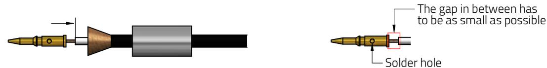
**Step 4.** Push cable with center contact into connector main body until perceptive point. Cover cable braid over connector neck carefully
